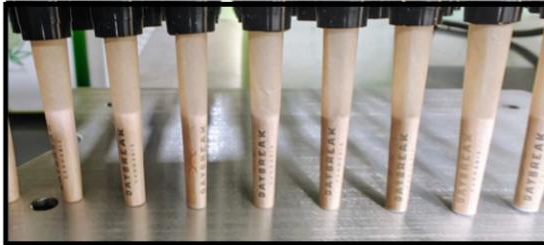
The Lift Plate levels cones from the bottom up for a more even fill line and accurate weights
