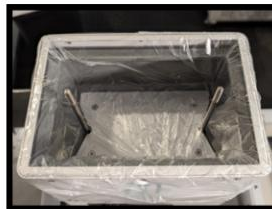
Tuck excess bag at the bottom underneath the Lift Plate.
